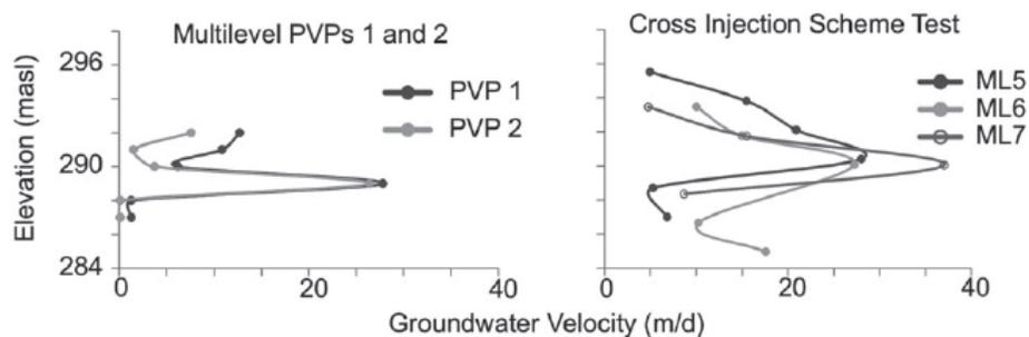
**Figure 7.** Depth versus groundwater velocity highlighting the preferential flow pathway transporting water at velocities observed by both PVPs and bromide tracer testing (bromide introduced by the cross-injection scheme, which flushes a zone between two wells oriented perpendicular to the ambient flow direction, modified from Schillig *et al.*, 2016).
