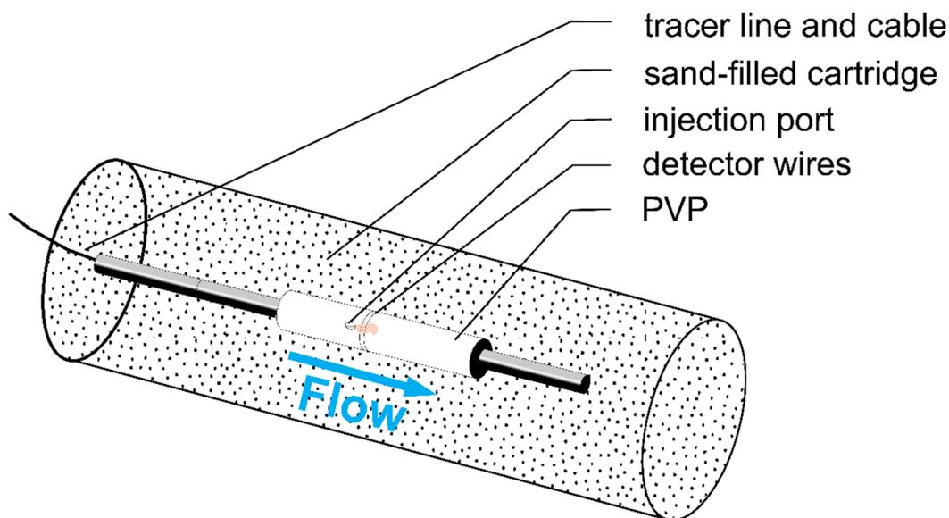
**Figure 3.** Schematic of the HRX-PVP within a sand-filled cartridge illustrating tracer (red) movement across the surface of the probe and detection wires. Modified from Cormican *et al* (2021).
