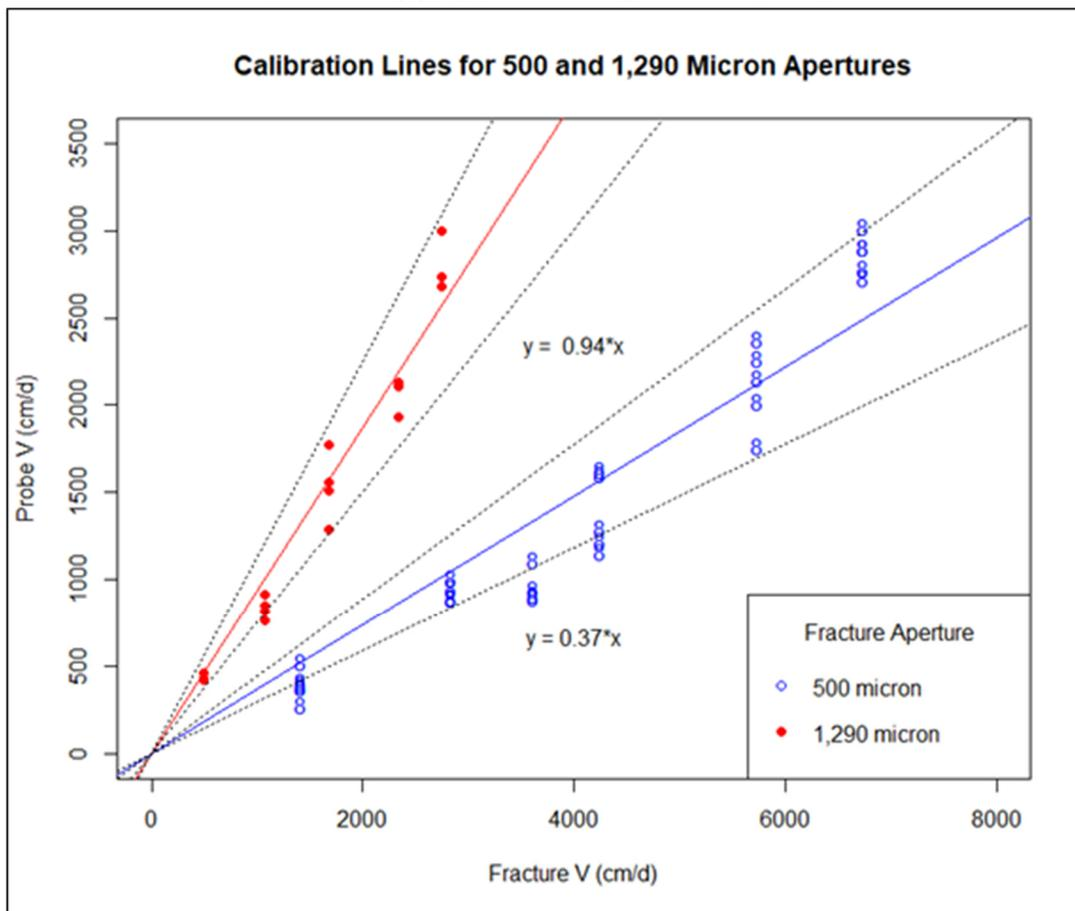
**Figure 14.** Linear relationship between measured F-IWPVP velocity and calculated water velocity through the fracture flow apparatus for two fracture apertures. The dotted lines indicate  $\pm 25\%$  error on calculated slopes.
