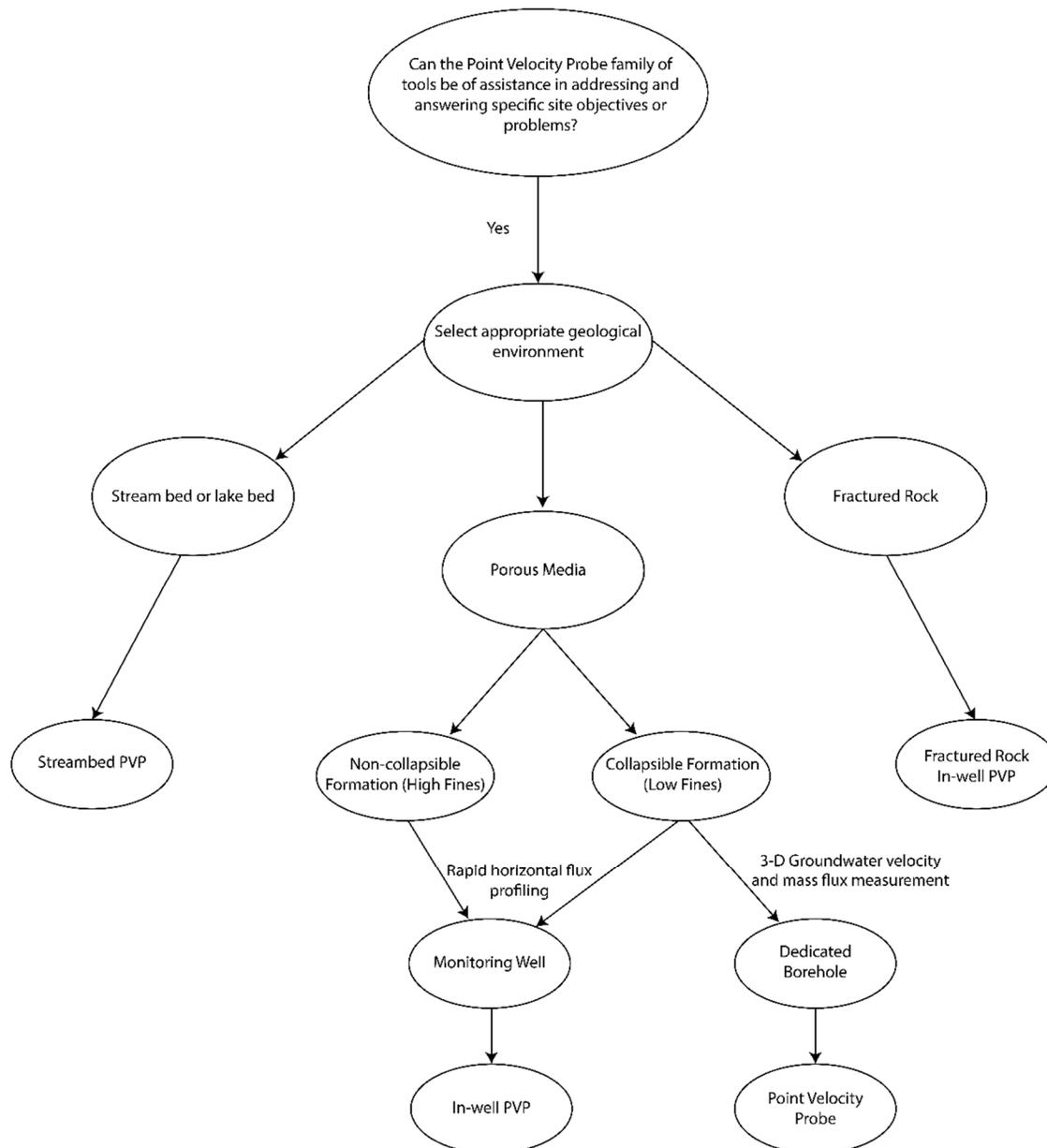
**Figure 1.** Decision tree for the selection of the appropriate Point Velocity Probe tool based on the geological setting of the study site.
