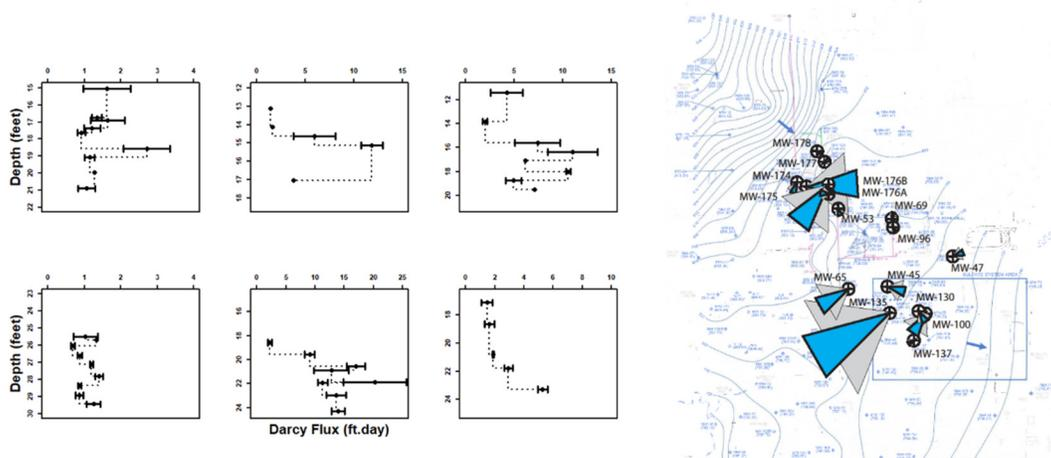
**Figure 13.** IWPVP depth versus flux profiles (left) for six of the 16 wells sampled throughout the four-day field campaign. The average flow behavior of the 16 wells sampled plotted on the water table contour map (right) allows for easy visualization of high and low flow zones as well as areas where IWPVP measurements highlight areas requiring further investigation to understand discrepancies between measurement methods. Modified from Osorno *et al* (2020).
