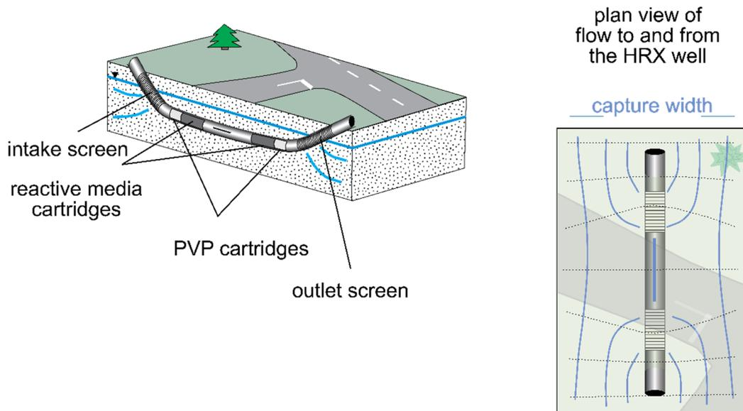
**Figure 10.** Schematic of the HRX Well<sup>®</sup>, left, showing the locations of the two HRX-PVPs installed at the upgradient and downgradient ends of the treatment section of the well. Estimates of groundwater velocities from the HRX-PVP were used to verify the passive capture of groundwater by the HRX Well<sup>®</sup>, illustrated in the plan-view schematic of the flow system, right. Modified from Cormican *et al* (2021).
