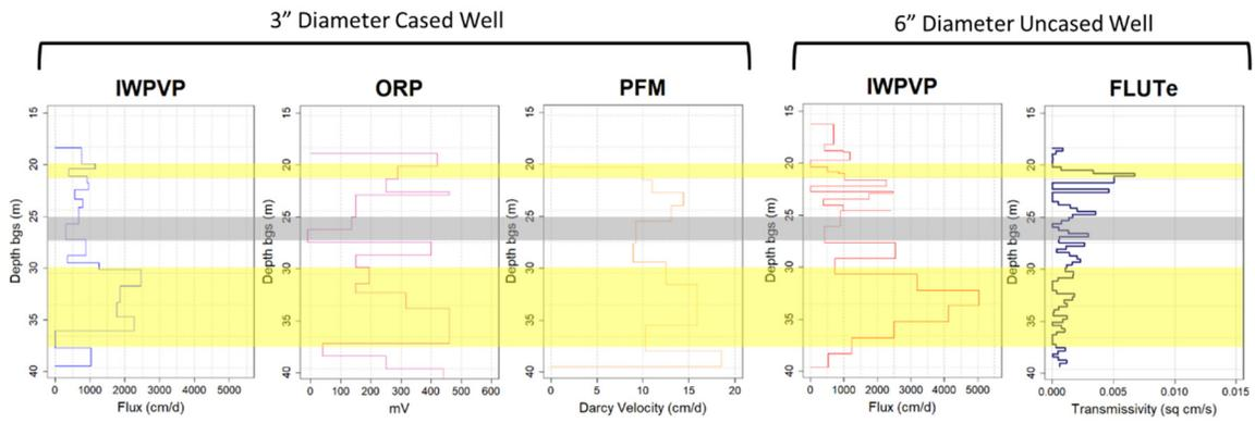
**Figure 15.** Comparison of depth profiles for all methods deployed in the two boreholes profiled at Edwards Air Force Base. Highlighted areas indicate similar trends of rate of flow with depth between profiles (yellow indicates areas of high flux and gray indicates areas of low flux). Modified from Heyer *et al* (in preparation).
