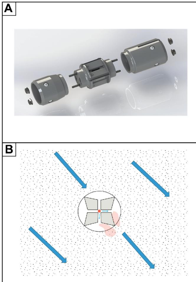
**Figure 5.** (A) Computer rendering of the updated modular IWPVP co-design by Solinst, the University of Kansas, and OUL. (B) Plan view schematic of the IWPVP illustrating tracer (red) movement through two measurement channels.
