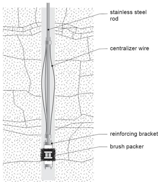
**Figure 6:** Schematic view of an F-IWPVP in a borehole showing the brush packers, reinforcing brackets, and spring-loaded centralizer wires. Taken from Heyer *et al* (in preparation).
