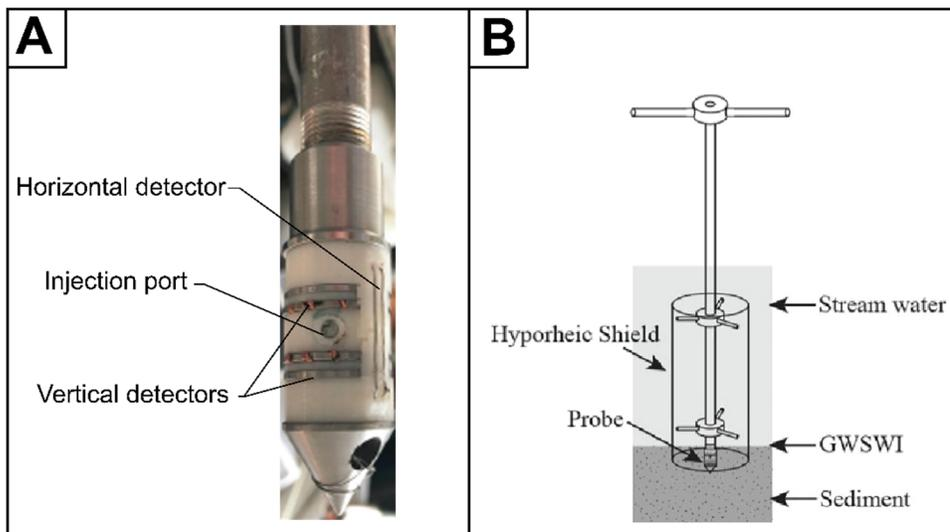
**Figure 4.** (A) photograph of the updated SBPVP with horizontal detection capabilities. (B) schematic of SBPVP deployment with the hyporheic shield for determination of vertical groundwater velocities at the groundwater-surface water interface (GWSWI) (modified from Cremeans *et al* (2018)).
