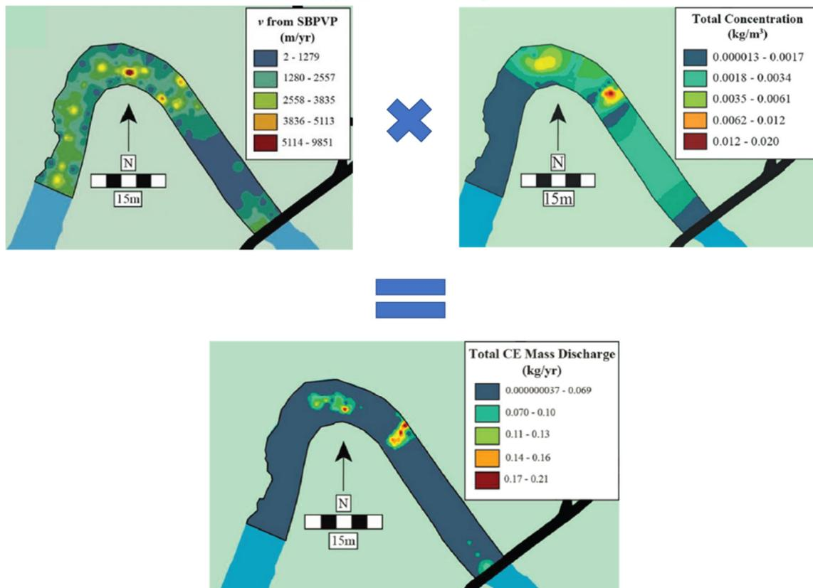
**Figure 11.** Distribution of vertical groundwater velocity (upper left) and aqueous concentration of chlorinated ethenes (upper right) along the study section of the meandering stream. The product of the two distributions, contaminant mass discharge (bottom center), highlights the discrete zones of high contaminant movement through the streambed into the stream. Modified from Cremeans *et al* (2018).
