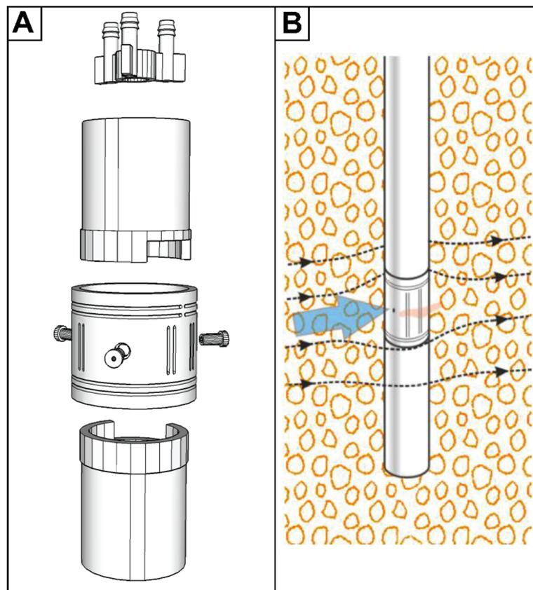
**Figure 2.** (A) Computer rendering of the PVP components and design. (B) Plan view schematic of the PVP illustrating tracer (red) movement across the surface of the probe and detection wires.
