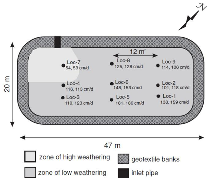
**Figure 12.** Plan view of the VFBR cell, showing the SBPVP sampling locations and estimated downward seepage velocities through the substrate. Taken from Cremeans *et al* (2019).
