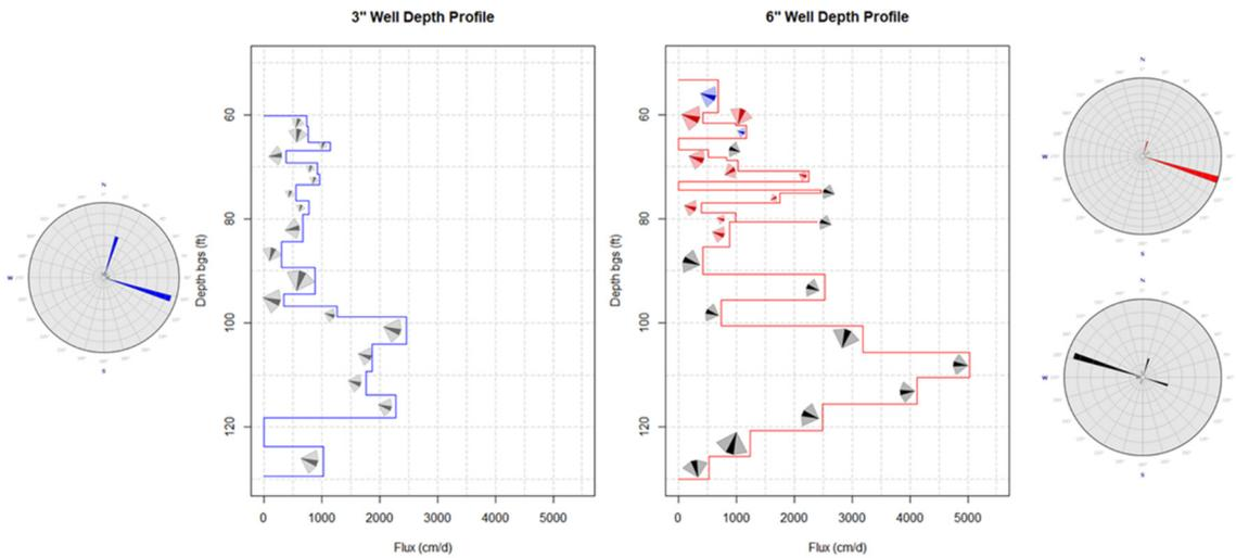
**Figure 16.** Depth profiles of F-IWPVP measured fluxes for the two boreholes profiled at Edwards Air Force Base. Rose diagrams show the general flow direction trend for each borehole. The blue and red rose diagrams refer to pre-rain event conditions and the black rose diagrams refer to post-rain event conditions. Modified from Heyer *et al* (in preparation).
