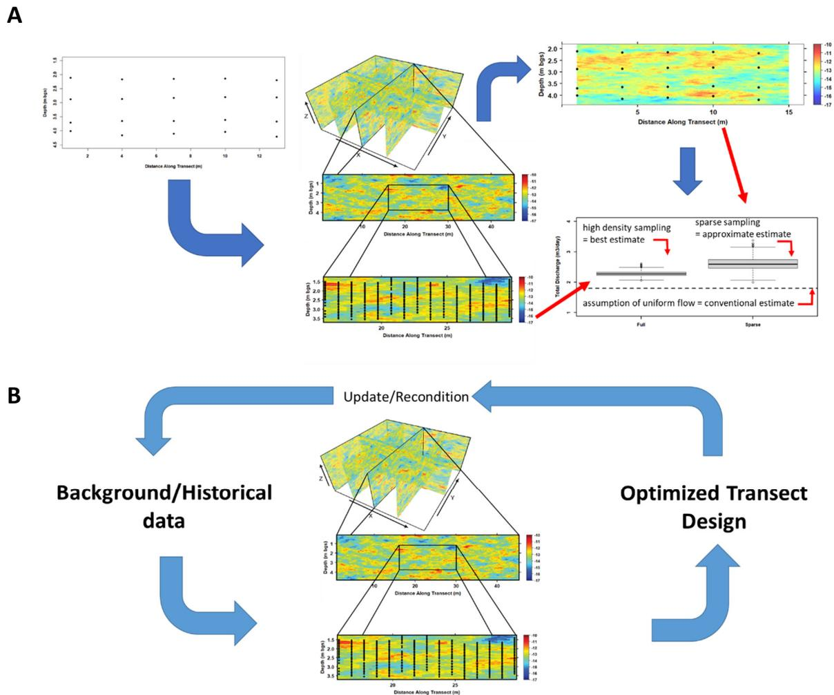
**Figure 9.** Conceptual work flow of optimized groundwater velocity transect design. (A) Workflow process for determining the lowest sampling density required while maintaining estimates of groundwater discharge within  $\pm 10\%$  with 50% confidence at the C.F.B. Borden study site. (B) Workflow process for development and refinement of transect design to achieve acceptable outcome levels *a priori*.
